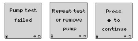
If () is not pressed or the pump is not removed within 25 seconds, the detector performs the pump test again.
