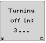
At the end of the countdown the detector emits an extended beep and flash, and displays 0 before deactivating.
