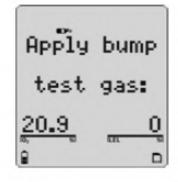
Note If the bump test is not performed, the detector deactivates.
