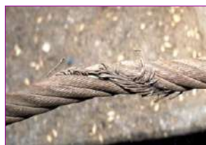
Wire rope wear
