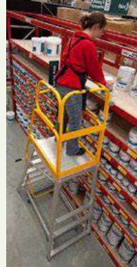
a worker uses a step platform with barriers on all sides.
