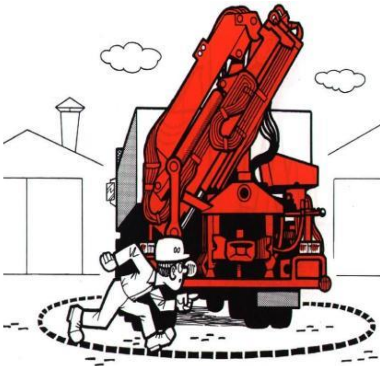
Check clearance around the crane
