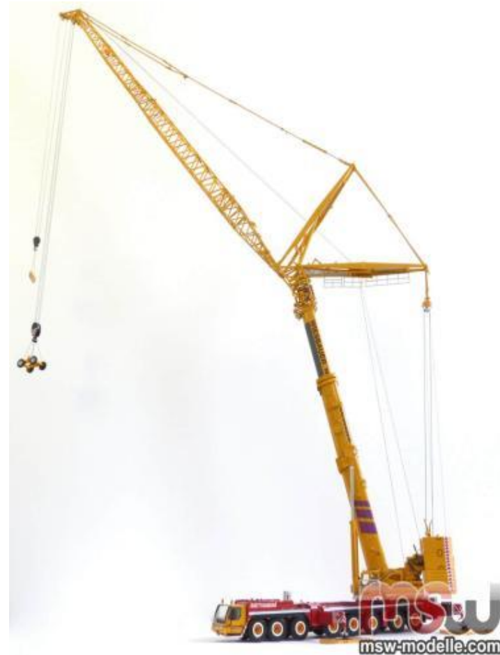
Telescopic jib fitted with latticed extension & fly jibs
