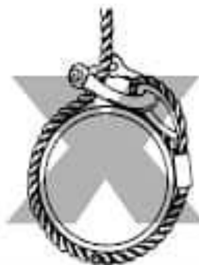
BAD – Bolt on running line can work loose
