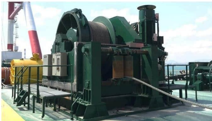
Mooring / Anchor Winch
