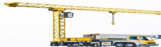
Mobile Tower Crane
