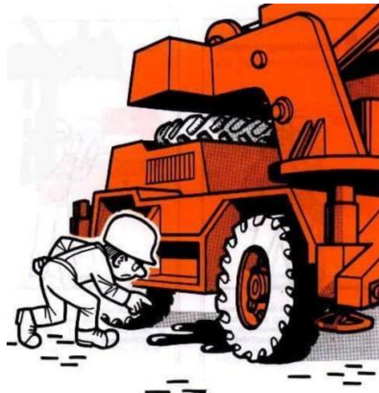
Remove all dusters, oil, grease, mud ...etc. To avoid fire initiation
