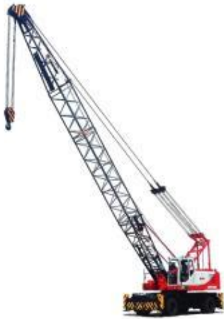
Latticed cantilever jib
