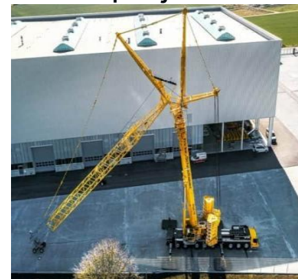
Telescopic jib fitted with lattice extension & fly jibs
